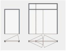
From single acting single doorsets to double acting double doorsets with overpanels and anything in between, we can configure your doors to suit your needs.
