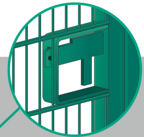
Padlockable Slide Bolt Detail
