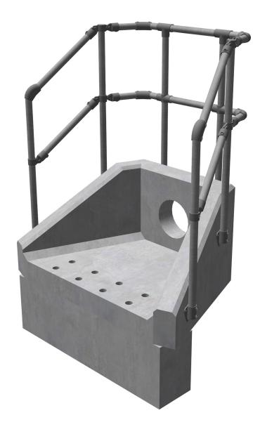
We are able to cast onto the apron of the basin inlet headwalls stepped baffle blocks for when the velocity of the discharge needs to be dissipated before it enters the watercourse.
