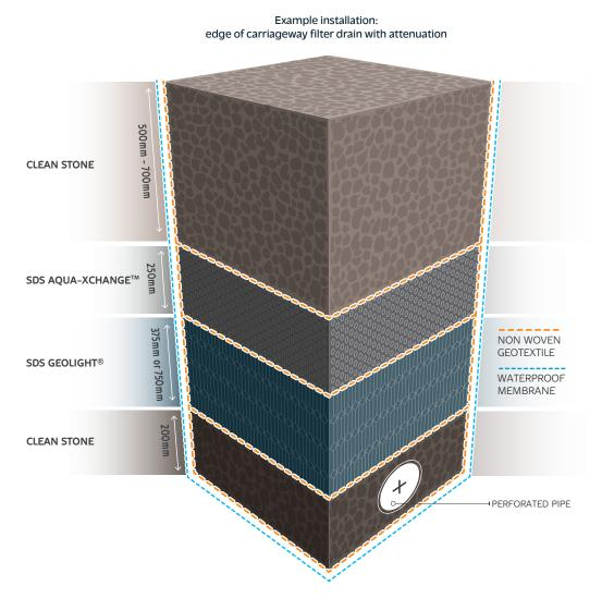
SDS Aqua-Xchange $^{TM}$  is a granular material suitable for use in devices where stormwater can percolate through the material, allowing sufficient contact time for the pollutants to be captured.
