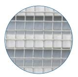
Material: Galvanised steel (stainless steel option available) Wire diameter: 1.5 mm Aperture: 12.7 mm x 12.7 mm Finish: Unfinished as standard Weight: 0.37 kg/m<sup>2</sup> Open area: 76% Louvre airflow reduction <sup>1</sup>: up to 5% Stock size: 1220 mm wide x 30 m long roll
