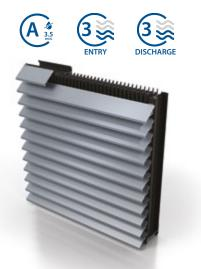
Airflow Coefficient C<sub>e</sub> (entry) 0.294 Airflow Coefficient C<sub>d</sub> (discharge) 0.299 Blade Pitch (front) 75 mm
