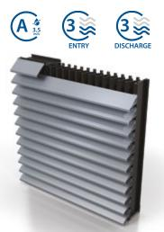
Airflow Coefficient C<sub>e</sub> (entry) 0.260 Airflow Coefficient C<sub>d</sub> (discharge) 0.232 Blade Pitch (front) 75 mm
