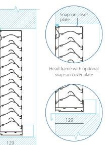
Cill frame with optional snap-on cover plate and typical cill pan (size to project requirements)
