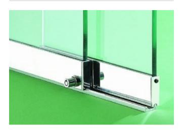
The usual overlap allowed between the two glass doors is 26 mm. For glass cutting sizes deduct 45 mm from the height of the opening.
