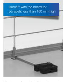
A toe board is required if a roof parapet is not present or is extremely low, with a height of less than 150 mm.
