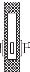
H3 ASSA 3088 deadlock (normally locked locations only) Euro cylinder outside Euro cylinder or thumbturn inside
