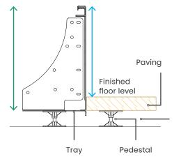
Minimum pedestal height: 20mm Standard 50mm Fire rated
