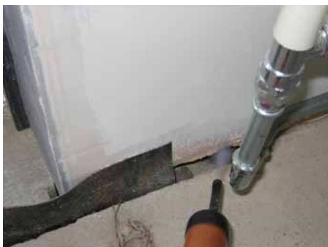
Figure 8.3 A smoke pencil (or 'puffer') being used to show air leakage through services penetrations. Picture courtesy of Kingspan.
