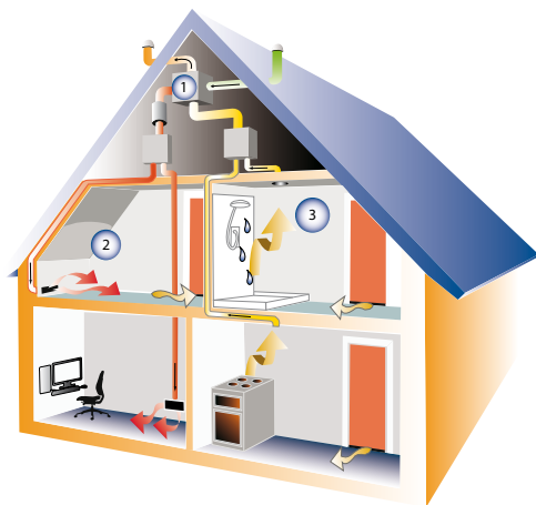
Figure 9.6 Whole house heat recovery ventilation. Warm air from wet rooms (3) passes through a fan and over a heat exchanger (1) where it heats incoming air delivered by another fan to living rooms and bedrooms (2). 19
