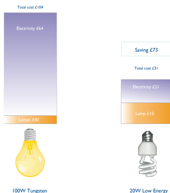
Figure 12.2 Even at a cost of £10 the compact fluorescent lamp saves seven times its cost over its life
