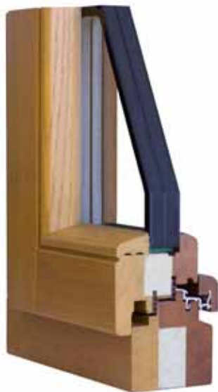
Figure 7.5 Triple glazed low emissivity gas filled glazing with insulated spacers in insulated timber frame, giving a whole window U value of around 0.75 W/m²K (Green Building Store)
