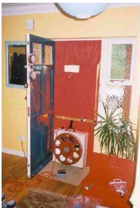
Figure 8.2 Pressure testing equipment. Picture: Rickaby Thompson Associates.
