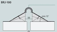
Flexible bellows incorporating a rubber membrane supported by a closed cell foam
