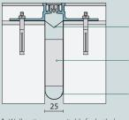
RFX-2F INSTALLED WITH ALS-200 FLOOR JOINT COVER
