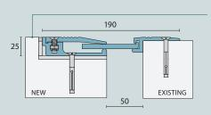
FFL at this point should be 6mm higher than the existing floor level.
