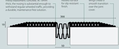
High strength epoxy bond holds up under constant deflection and temperature extremes.
