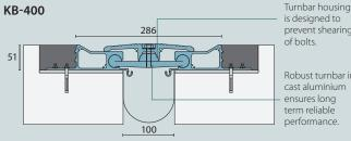
is designed to prevent shearing of bolts.
