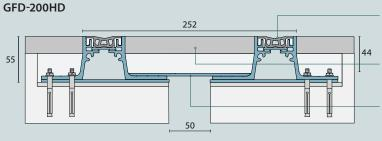
Smooth TPR gaskets are suitable for areas where hygienic finish is required. They are installed with a continuous aluminium support plate underneath for added durability.
