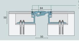
Exposed sections are serrated for a slip resistant finish.
