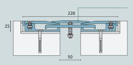
Secondary centre plate for increased durability and smoother transition in areas where trolley traffic is prevalent.
