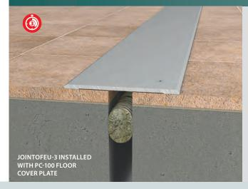
**EXAMPLE APPLICATION:** Jointofeu-3 used in conjunction with PC-100
