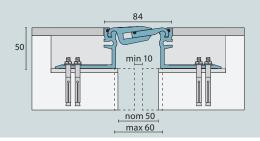
APF models can be installed over a range of joint widths, or over uneven joint widths, whilst still maintaining the same movement capability.
