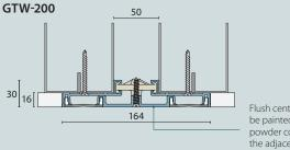
Flush centre plate can be painted or supplied powder coated\* to match the adjacent wall finish.
