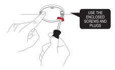
Once the mounting base is installed, attach the alarm by twisting clockwise until it clicks. If
