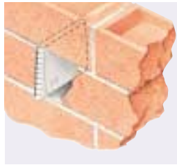
Cranked sleeve+integral cavitytray
