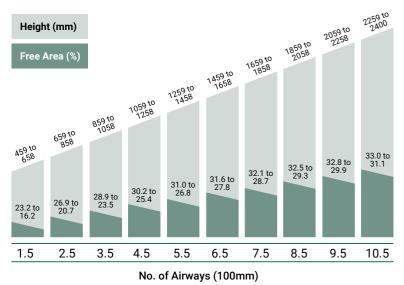
Free area and pressure drop shown is based on a 1150mm wide single piece louvre fitted with bird mesh and will vary slightly for different widths and larger heights. Pressure losses for Class A rated louvres and/or Insect mesh are available upon request.
