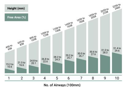
Free area and pressure drop shown is based on a 1150mm wide single piece louvre fitted with bird mesh and will vary slightly for different widths and larger heights. Pressure losses for Class A rated louvres and/or Insect mesh are available upon request.
