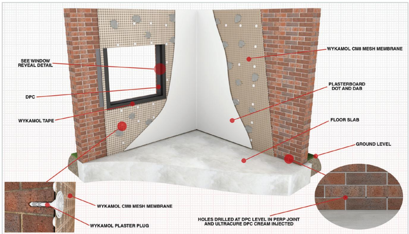
Plasterboard should not be directly fixed to walls with a history of dampness issues using traditional gypsum adhesive as this may result in visible damp patches where the adhesive acts as a bridge for moisture or salts between the old masonry and the plasterboard surface.
