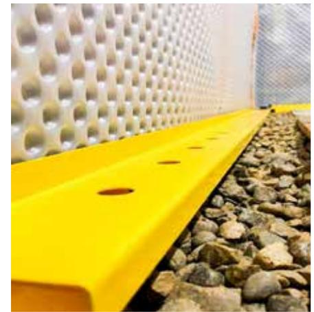
The concept of a Drained Cavity System is to collect and manage any ground water which breaches the integrity of a structure by managing, collecting and discharging such free water via a suitable evacuation point such as a Delta Packaged Pump Station.
