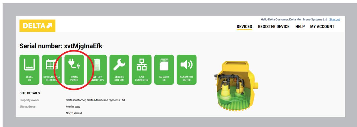
Figure 23b. An example of the Delta Pumps App dashboard showing mains power present.
