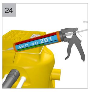
Once chamber has been filled with water, apply Delta AKTI-VO 201 (swellable mastic) to the entire external lip locator of chamber.
