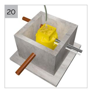
Completely fill chamber with water.
