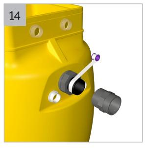
Wrap the thread on the tank connector's male thread with with PTFE tape.
