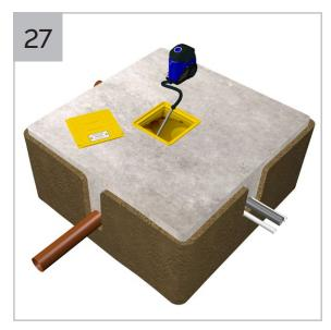
Once successfully installed all chambers should be emptied. Use of temporary site pump(s) are suitable for this exercise. Care should be taken in ensuring water is being discharged somewhere suitable.
