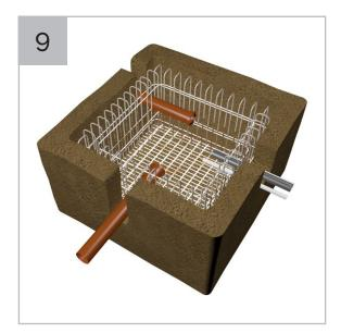
Lay inlet and discharge pipework. Allow pipework to protrude into cage by a minimum of 100 mm.
