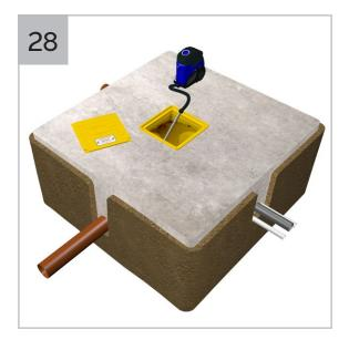
Manually remove any debris from chamber and residual water using a wet vacuum.
