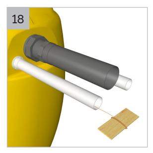
Ensure a draw cord is pulled through the cable duct as the cable duct is built.
