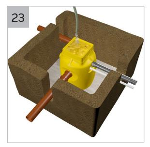
Completely fill chamber with water.
