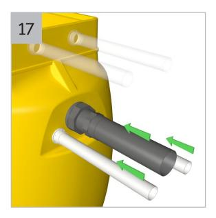
Push discharge and cable duct pipe into their respective fittings, twisting the pipe as it is pushed in to remove any trapped air.
