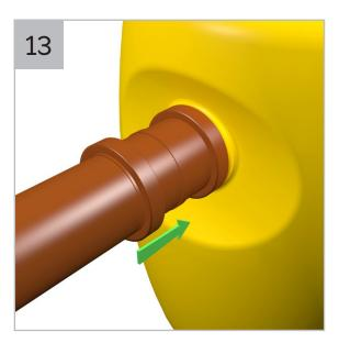
Connect inlet pipework to the chamber spigot.
