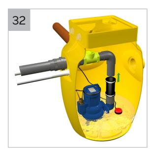
Push pipe into the rubber drain coupling.
