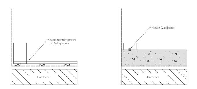
Koster Quellband should be included in the applicable slab construction joints.
