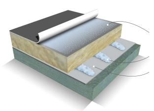
Bonding fleece-backed synthetic roofing membrane to insulation.
