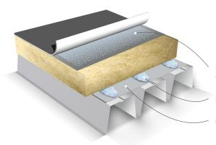
Bonding fleece-backed synthetic roofing membrane to insulation.
