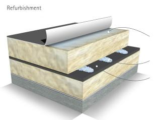
Bonding fleece-backed synthetic roofing membrane to insulation.
