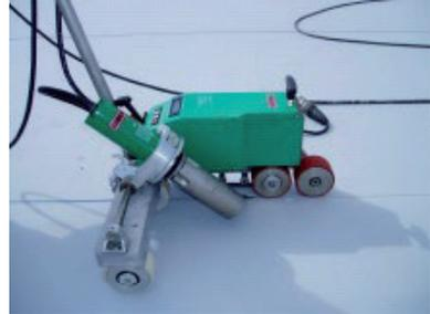
The air supply filter must be clear and free from dust. Accumulated dust and dirt are to be removed using a brush or compressed air.
