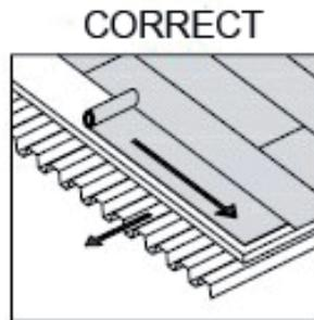
Screws and pressure plates are installed on the side lap. A marker line has been applied for this purpose.
