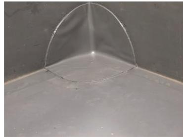
Hot air weld with a 20 mm nozzle in combination with a penny roller.
