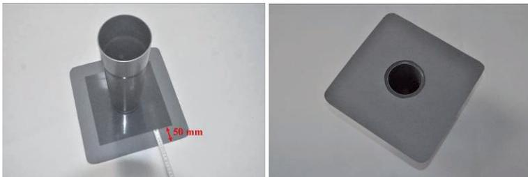
Weld the flange by hand to the prefabricated outlet by means of hot air (20 mm wide nozzle) or solvent weld. Keep a weld-free area in the four corners for mechanically fixing the rigid plate to the upstand or deck.
