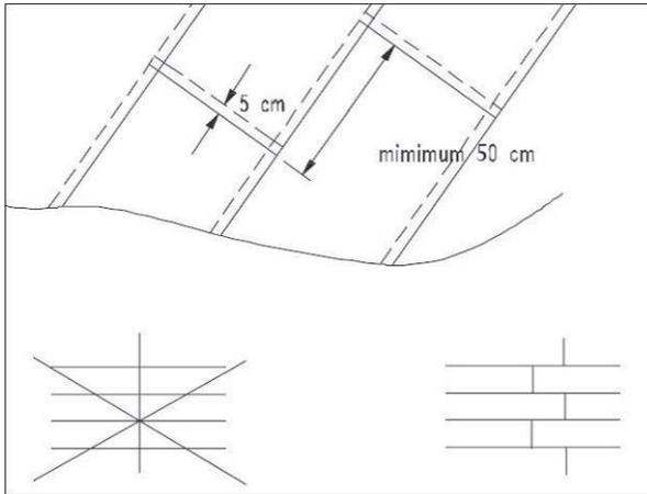
End laps from the end of the roll of **RENOLIT** ALKORPLAN roofing membrane must be cleaned to remove any tape or adhesive used in the rolling of the membrane and then must be overlapped by 50 mm and welded in the normal way. The end joints across the roof must be staggered to give a minimum of 500 mm between each joint.
