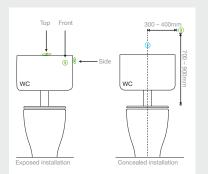
The cistern is supplied with the **easyflush** valve already installed inside it. The installer only needs to connect to the water supply and pan. To install and commission there are three easy steps:
