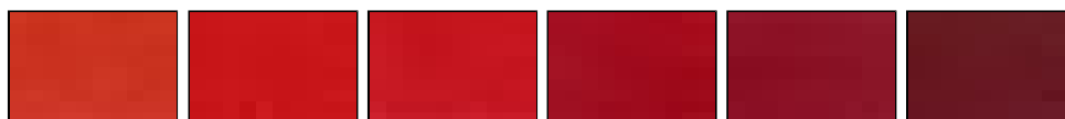
3000 Flame Red 3001 RAL Signal Red 3002 Carmine Red 3003 Ruby Red 3004 Purple Red 3005 Wine Red
