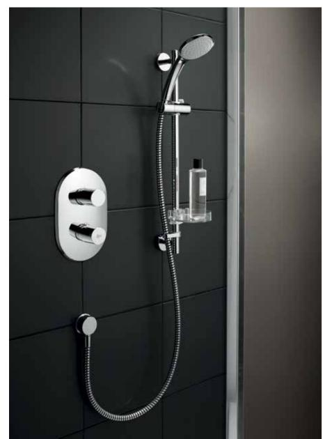
Innovative and practical, this shower mixer boosts water flow in low pressure areas. Using the Venturi principle, the Boost increases hot water flow rate by harnessing the energy in high pressure mains cold water.
