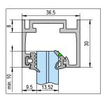
🚺 Glass thickness tempered glass 8 - 12 mm, laminated glass 8.76 - 13.52 mm · Please order corner connectors and sealing strips separately, depending on the glass thickness · Work length 4950 mm
