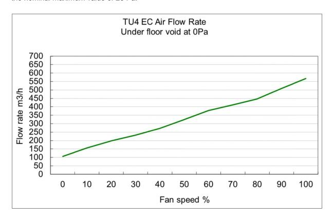
In the reading of the air flow value it must be considered that in a typical installation the under floor static pressure in the supply zone is normally between 3 and 15 Pa.
