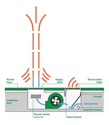
Note: Approximately 5% air flow reduction must be considered when the TU4 is fitted with the optional electric heater.
