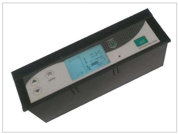
With the LCD controller, all programming setup and modification of the working parameters are carried out using the controller's four push buttons as indicated in the image above. The functions available depend upon the TU4-EC configuration; please refer to the Fatronic user manual for full information.
