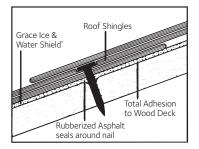
Seals around nails or fasteners. Fully adheres to deck, resisting leaks from wind driven rain or water backup due to ice dams.
