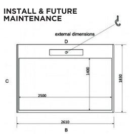
Hook in the building ceiling for 500kg, by builder, centred over guide frame. (Can be removed after installation.)
