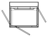
Configure your lift with doors on up to 3 sides over the whole travel of the lift.
