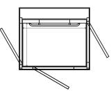
Configure your lift with doors on up to 3 sides over the whole travel of the lift.
