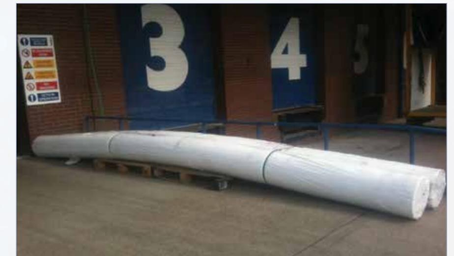
These super-jumbo rolls are designed for use for very large projects, such as road construction, reservoirs and landfills. Using very wide rolls reduces the number of joints between individual rolls. This cuts down on labour by having less individual rolls to stitch together, and also makes the whole fabric layer stronger by having less weak points at the joints.
