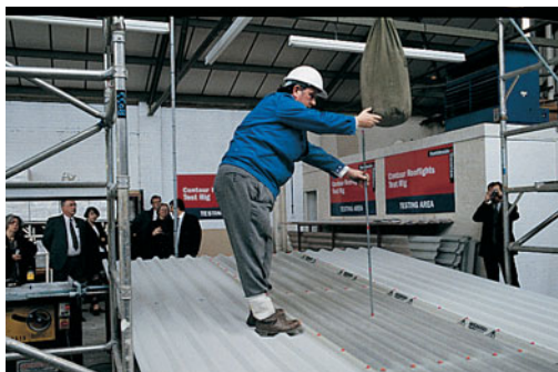
Measuring the height of 1.2 metres for the first drop in the test sequence on StepSafe.
