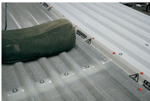
StepSafe after two drops from a height of 1.2 metres.
