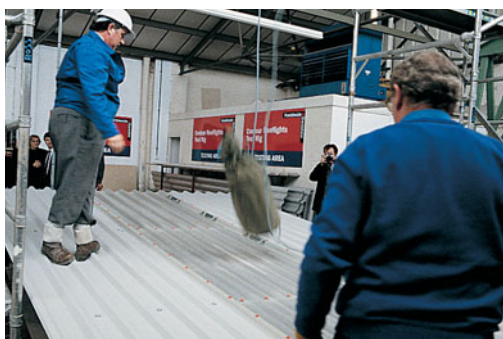
A 45 kg bag freefalls from a height of 1.2 metres before impacting on StepSafe in the second drop of the test sequence.
