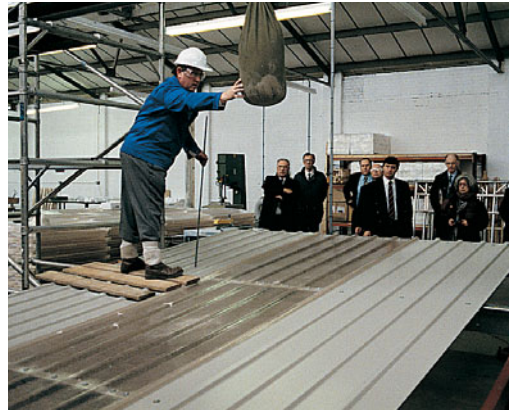
Lining up for the first drop on to the unfixed and untaped side laps of the Contour Class 1 fire rated Liner Panel 2.44 kg/m 2 from a height of 1.2 metres.
