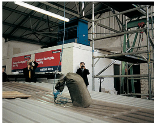
After the second drop in the test sequence from a height of 1.2 metres the Contour Liner Panel shows minimal deflection.
