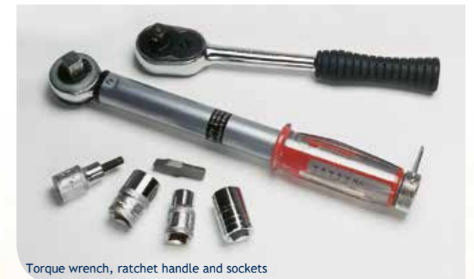
4. Evenly tighten the bolts to the required torque setting. The coupling should only be tightened once, because it cannot be dismantled and re-used. (See Couplings Data page 55)
