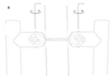
Suitably line the holes up to where the handle will be fitted on the door making sure it is straight.
