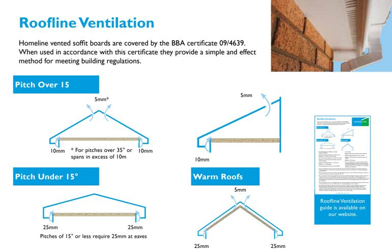
Single vented boards offer a 14mm continuous slot or 14,000 square mm pre linear metre, with double vented boards offering a 28mm continuous slot or 28,000 square mm pre linear metre.
