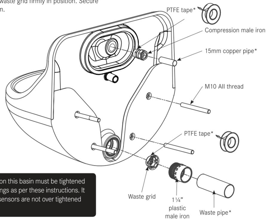
**IMPORTANT :** The fixings on this basin must be tightened to the recommended settings as per these instructions. It is also important that the sensors are not over tightened during Step.5.
