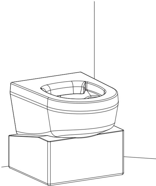
Using the cradle, slide the pan in to place against the wall so all the fixing studs protrude through in to the service duct.
