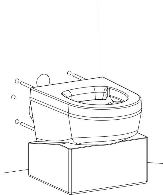
Screw the M12 studding into the back of the pan as far as possible. Make sure a flush pipe cone and outlet connector is fitted in the back of the pan. The cradle can be used to support the pan. Align the pan with fixing holes.
