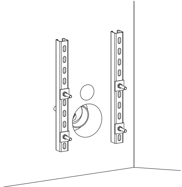
Secure the pan using the nuts and washers supplied- tighten using a torque wrench to 22-24 Nm. Connections to the WC flush pipe and soil pipes are conventional.
