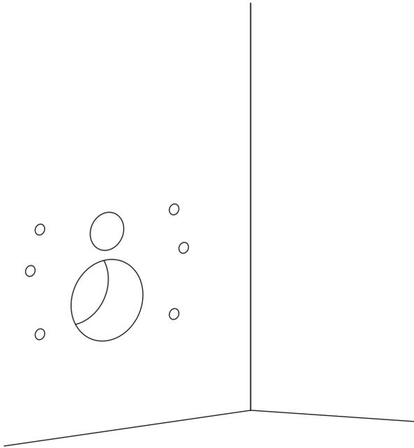
Use the drilling template provided, mark and drill holes for the inlet, waste and fixing studding. For disabled use, raise hole heights an additional 60mm.
