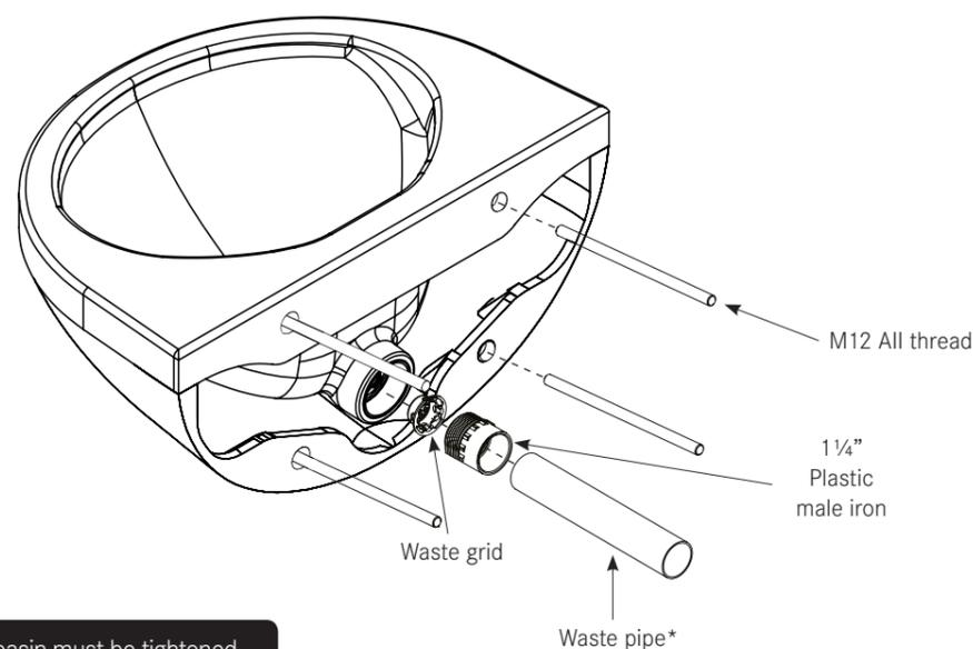
**IMPORTANT :** The fixings on this basin must be tightened to the recommended settings as per these instructions.
