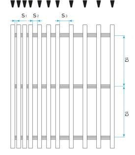
S = Slot spacing tQ = Variable support profile spacing
