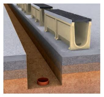
The installation of the channels shall be started at the evacuation point or at the deepest point.
