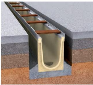
Before tipping out the concrete for the concrete bedding place wooden battens or the gratings themselves protected with plastic, in order to prevent deformations which might impede the placement of the gratings.
