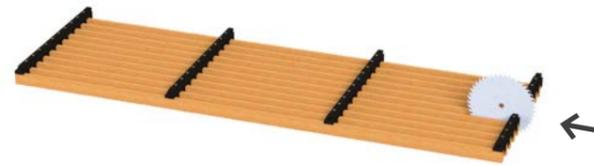
Step 3: Male cut finish – Screw on the edging strip (option) – Pre-drill Ø 2 mm
