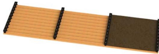
Step 3: Fix the particle plate on the slats and draw the outline
