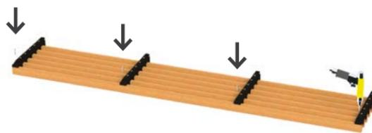
Step 7: Screw on the edging strip (option). Pre-drill Ø 2 mm
