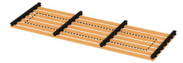
Step 2: Cut the panel at the position marked
