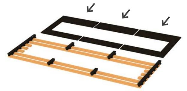
Step 5: Fix the particle plates on the slats
