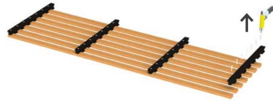
Step 3: Screw the cutting profile in the position marked
