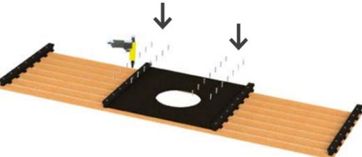
Step 6: Add the mineral wool tiles, the panel is ready to be fitted
