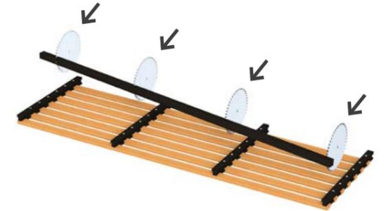
Step 3: Screw on the profile to hold the slats
