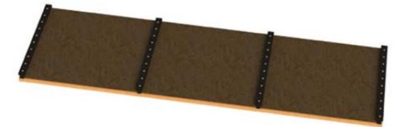
Step 3: Fix the particle plate on the slats and draw the outline
