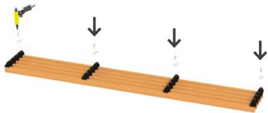
Step 4: Female cut finish – Unscrew the slat-retaining screws
