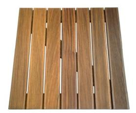
Pre-assembled 500x500 mm, 30 mm thick deck tiles in lpè wood, each made up of seven 15x67x500 mm boards, to create an anti-slip flooring surface, and three 15x67x500 mm battens for the substructure, positioned in a "Z" formation.
