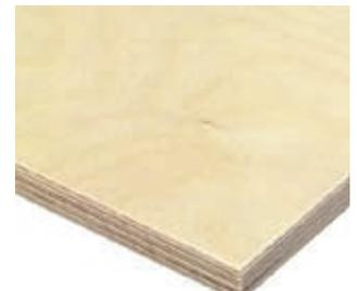
*The standard veneer thickness for most European Birch plywood is 1.4mm. Plywood normally has a balanced construction of alternating cross and long grain veneers, i.e. 9-ply for 12mm, 13-ply for 18mm.*
