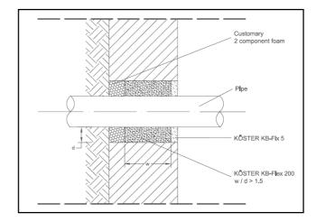
Before applying KÖSTER KB-Flex<sup>®</sup> 200, a securing block is installed in the penetration at a depth of 10 cm using a customary 2C PU-foam. The KÖSTER KB-Flex<sup>®</sup> 200 cartridge is then placed in the gun and the material is pressed into the penetration from back to front utilizing the flexible nozzle so that the resulting layer thickness is at least 8 cm.
