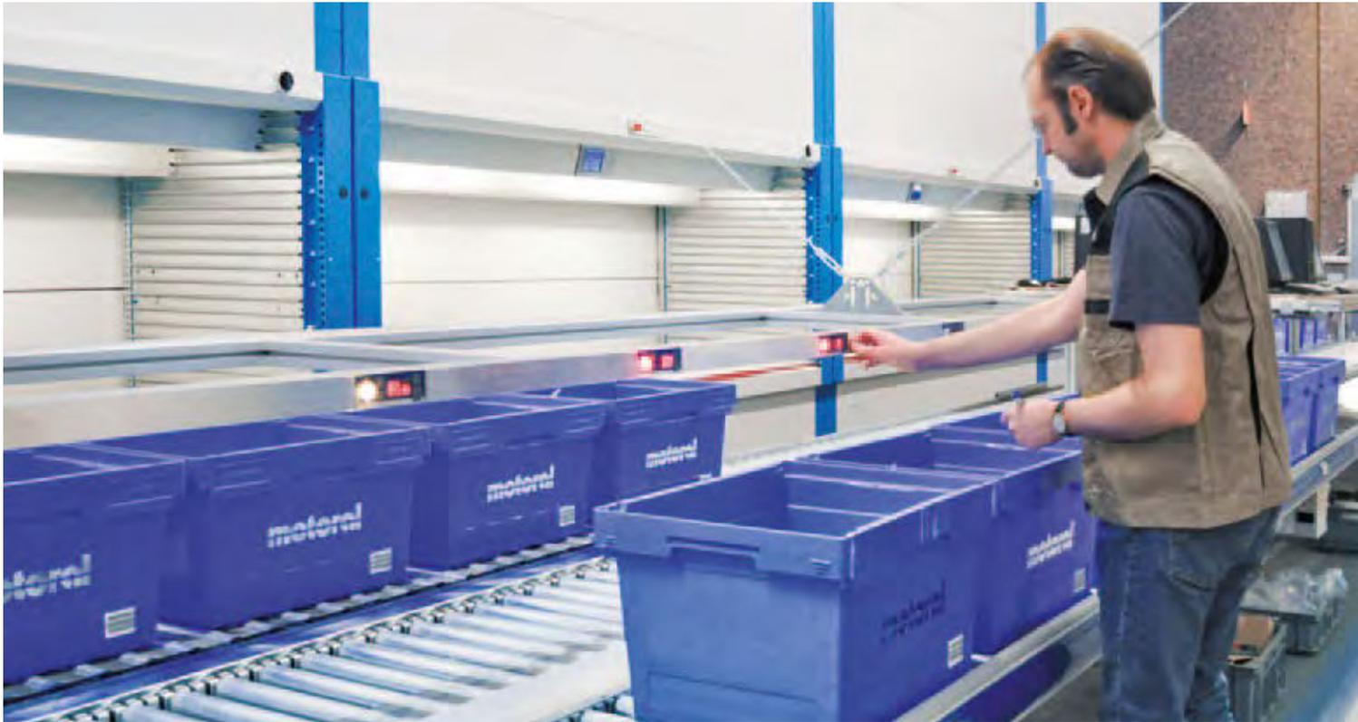
The amount of order picking locations and pick-by-light displays and the buffer capacity are determined by customer-specific demands.
