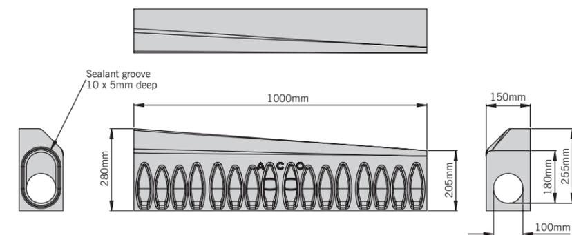
Note: For details regarding the gully, foul air-traps and drain unions for use with this system please refer to page 68. These products are subject to weight and dimensional tolerances. The dimensions shown on this page are for guidance purposes only.
