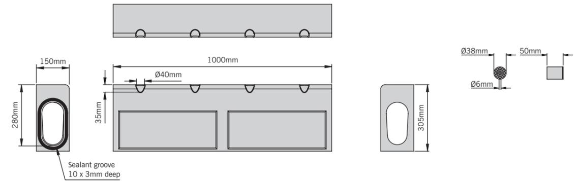
Note: For details regarding the gully, foul air-traps and drain unions for use with this system please refer to page 68. These products are subject to weight and dimensional tolerances. The dimensions shown on this page are for guidance purposes only.
