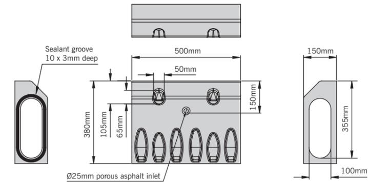
Note: For details regarding the gully, foul air-traps and drain unions for use with this system please refer to page 68. These products are subject to weight and dimensional tolerances. The dimensions shown on this page are for guidance purposes only.
