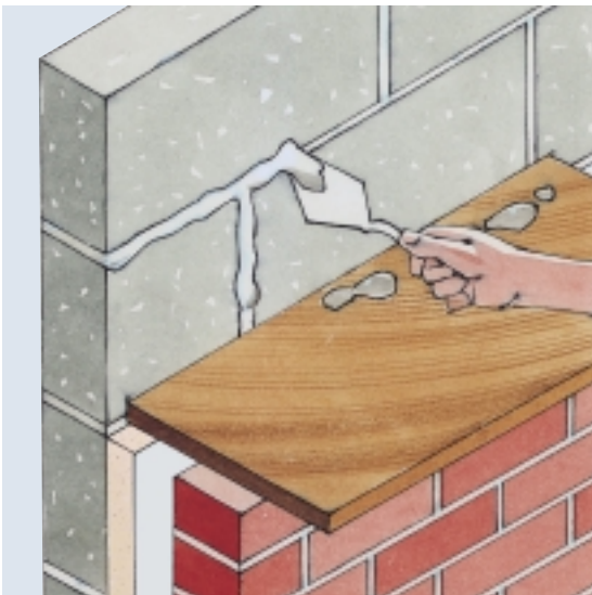
Figure 6 USE OF A CAVITY BOARD TO PROTECT THE CAVITY
