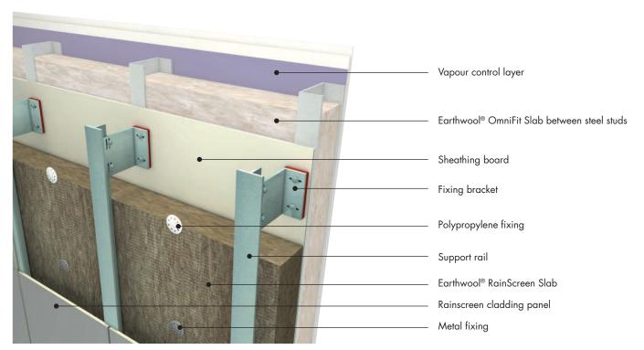
Note: Breather membrane can be used although not shown
