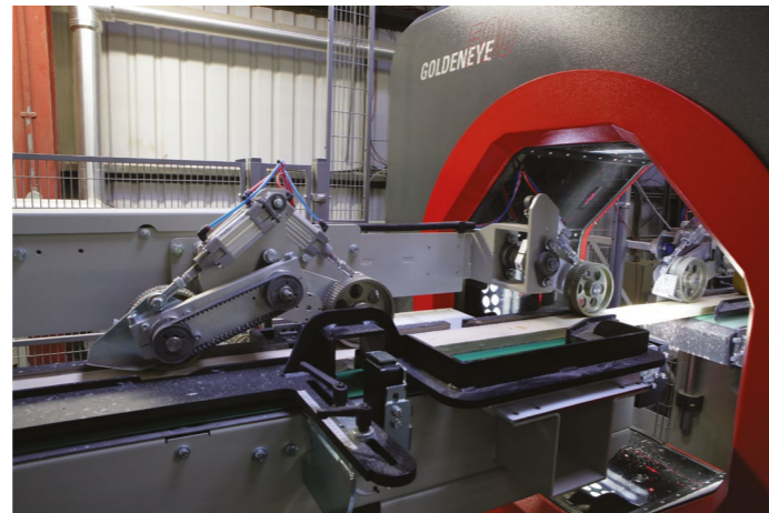
Goldeneye, roofing batten scanning line.
